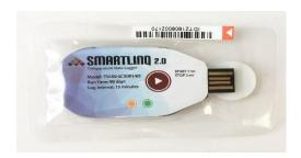
The one thing that **SMARTLINQ TDL temperature data loggers** all have in common is that they are very easy to use. The **SMARTLINQ TDL90 v2 data loggers** are controlled **with only one button**. Pressing this button for 3 seconds will start recording and the recording cycle will end when pressing this button for 3 seconds again.
