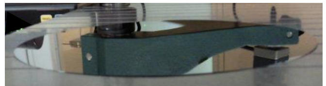
Fig.1 Warpage comparison of 50um thick wafers with 10um films
