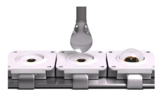
dispensing equipment or can also be compression molded using compression mold equipment.
