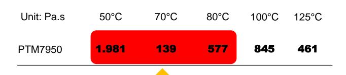
Invalid data due to high viscosity below 80°C. Sliding issue was observed between rotor and PTM7950
