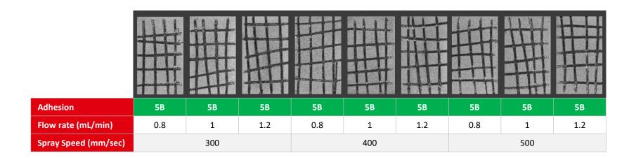
• All of the tested coating conditions provided 5B adhesion results.
