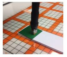
Uses 1GHz and 5GHz antennae and a real-time EM scanner (designed for EMI pre-compliance and diagnostics).
