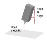
Spray Head Directions For 4 Sidewall Coverage
