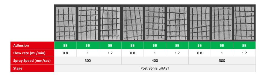
• All of the tested coating conditions passed adhesion at 5B after MSL3 + 96hours uHAST.
