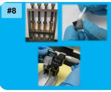
Take out the sample after 60min, room temperature to cool the samples for 20 min, clean up the sandwiched samples and test the thickness and measure the final thickness of sandwiched sample.
