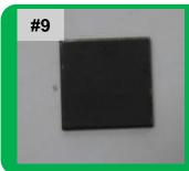
Spray the graphite spraying on both surface of sample with thin thickness, after the solvent dry out, test time zero TI with laser flash.
