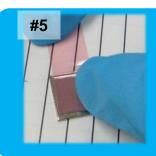
Paste one sample with size 10 x 10mm on the center of Cu plate, press it to stick on well and cover another Cu plate on the sample.
