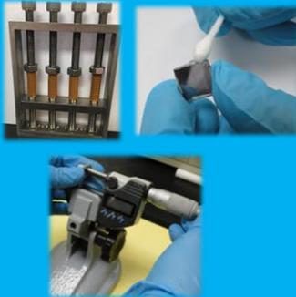
Take out the sample after 60min, room temperature to cool the samples for 20 min, clean up the sandwiched samples and test the thickness and measure the final thickness of sandwiched sample.
