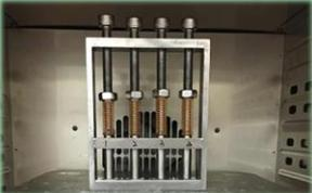
Take vertically the fixture with sample into 90C oven for 60 min.
