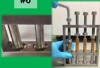
Put the sandwiched samples into the fixture with 35psi and fasten it.
