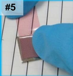
Paste one sample with size 10 x 10mm on the center of Cu plate, press it to stick on well and cover another Cu plate on the sample.
