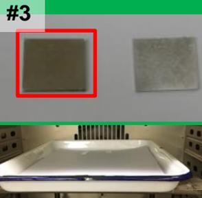
Clean the surfaces of Cu plate with EA, especially for the surfaces which contact samples, then put Cu plates into the 90°C oven for 5 min and cool Cu plates well.
