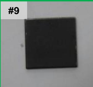
Spray the graphite spraying on both surface of sample with thin thickness, after the solvent dry out, test time zero TI with laser flash.
