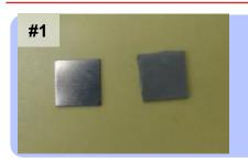
Select two pieces of Copper plates with known thickness. Standard PCM material (12x12mm, 0.25mm thickness) was pasted on one plate and covered with the other plate.
