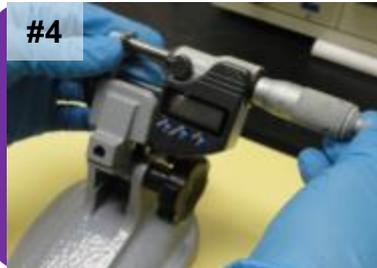
Measure the total thickness of the sandwich sample, and get the BLT data after calculation
