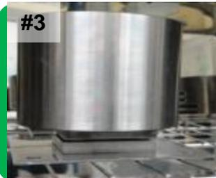
Put the fixture in 80'C oven and load 1~100PSI pressure on the fixture for 30mins
