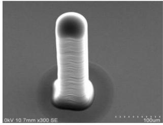
3.5:1 aspect ratio inkjet printed UV-cure polyacrylate (PA-1510 series)
