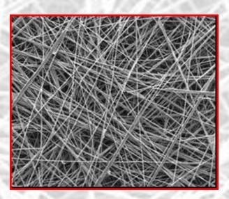
Spectracarb™ GDLs are produced in the USA and are available in a wide range of standard and custom grades, densities, sizes and materials for fuel cells, electrolyzers, humidifiers, specialty batteries and other electrochemical applications.
